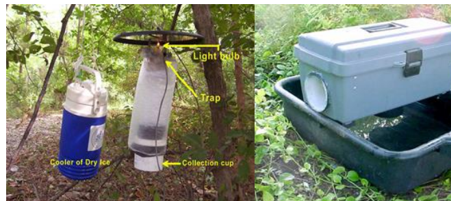
Above is an example of a BG Sentinel trap used by the health department for mosquito surveillance. Below is a CDC light trap on the left, and a Gravid trap on the right. If you see a trap, please do not disturb it.
