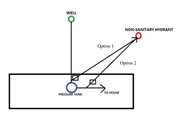
**Option #1** – Non-sanitary hydrants that are plumbed in water line before the pressure tank need a backflow device that meets ASSE 1024, 1015, or 1013 standards. A well alteration permit is needed for this connection if the well is existing and there is no permit already.
